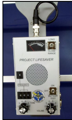
Project Lifesaver Mobile Digital Receiver Used By Law Enforcement to Locate Missing Person
